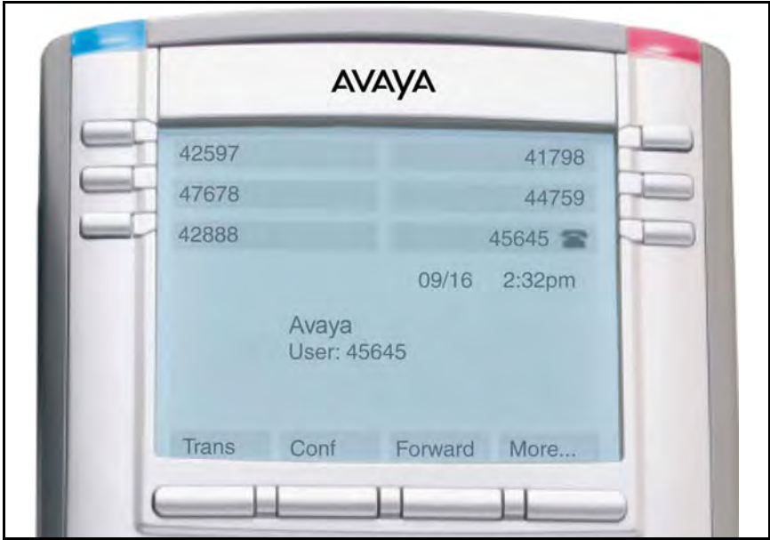
Figure 28: Logged in to an Avaya 1120E IP Deskphone using an Avaya 1140E IP Deskphone
